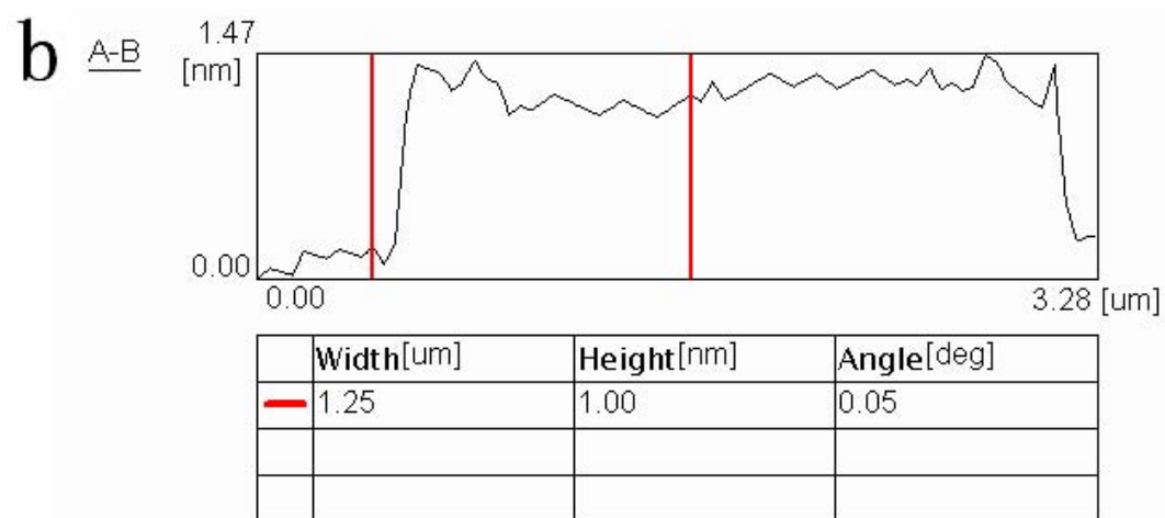
Fig.S4 (a) AFM image of GO; (b) cross-section analysis of GO
