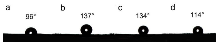
Fig. S3 Water contact angle over (a) HPA@SiO 2 ; (b) HPA@SiO 2 -S; (c) HPA@SiO 2 -S-N 2 ; (d) The HPA@SiO 2 -S-N 2 catalyst after reused for 5 times.
