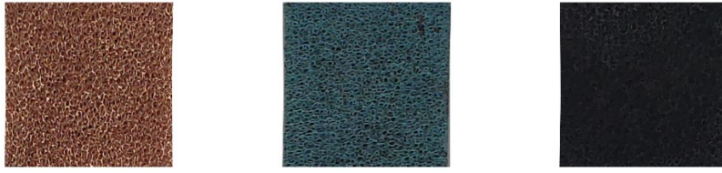
图 S1 空白泡沫铜(CF = Copper Foam)、 \text{Cu}(\text{OH})_2/\text{CF} 和 \text{Cu}_3\text{HITP}_2/\text{CF} 的光学照片(从左至右) Fig. S1 Optical photographs of Copper Foam, \text{Cu}(\text{OH})_2/\text{CF} and \text{Cu}_3\text{HITP}_2/\text{CF} (from left to right).
