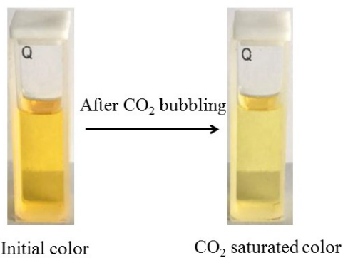
Fig. S4 The color change from orange to yellow after CO 2 bubbling in [P 66614 ][PhN=NPhO] CHCl 3 solution.
