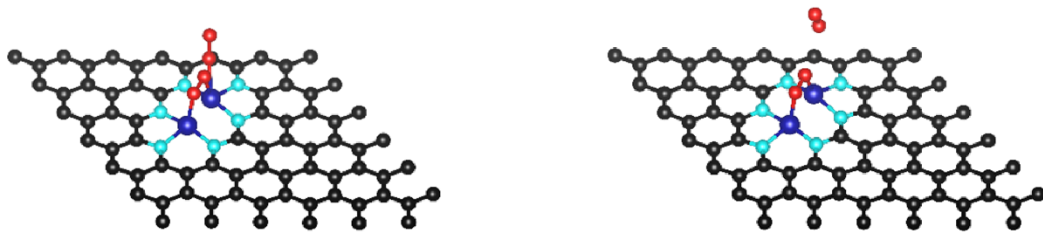
Fig. S8 The oxygen molecule adsorbs the configuration on Co 2 -type1 which pre-adsorbs one oxygen molecule (One O 2 is pre-adsorbed, and the second O 2 will not be adsorbed on Co 2 -type1).
